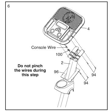
Slide the Console Cover (96) (see the drawing in step 6) upward to the Console (4). Attach the Console Cover with four M4 x 16mm Screws (84).
